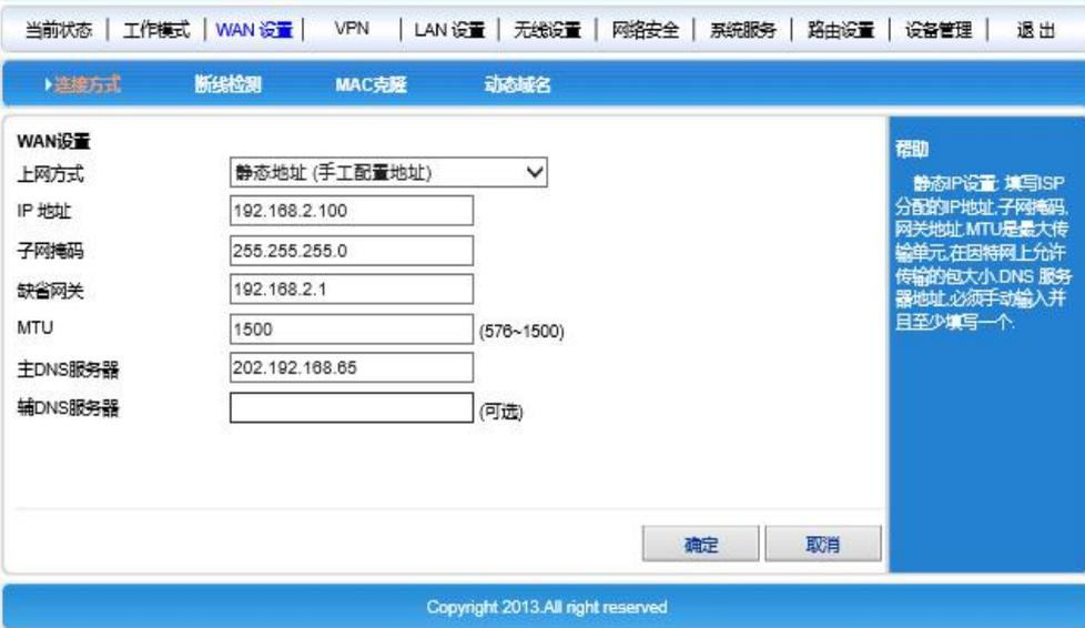
The screenshot shows the router's management interface in 'Work Mode' (工作模式) with the 'WAN Settings' (WAN 设置) tab selected. The 'Connection Method' (连接方式) is set to 'Static IP (Manual Configuration)' (静态地址 (手工配置地址)). The configuration fields are as follows:
