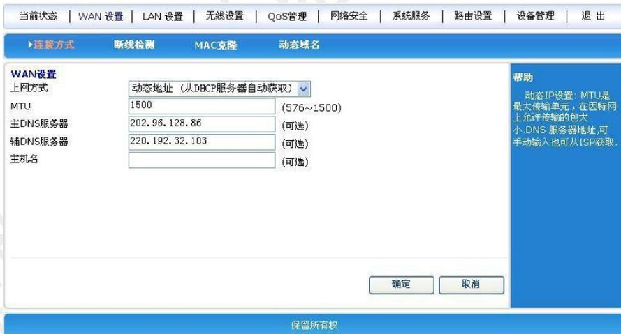
The screenshot shows the 'WAN 设置' (WAN Settings) page with '上网方式' (Internet Access Method) set to '动态地址 (从DHCP服务器自动获取)' (Dynamic IP (Automatic acquisition from DHCP server)). The configuration fields are as follows:
