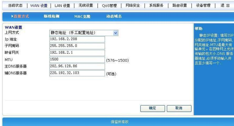
The screenshot shows the 'WAN 设置' (WAN Settings) page in the router's management interface. The '上网方式' (Internet Access Method) is set to '静态地址 (手工配置地址)' (Static IP (Manual Configuration)). The configuration fields are as follows:
